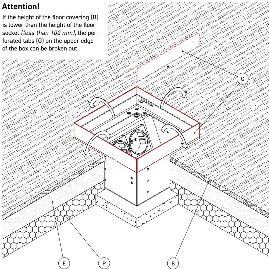
*Cross-sectional view with tabs broken out.*
